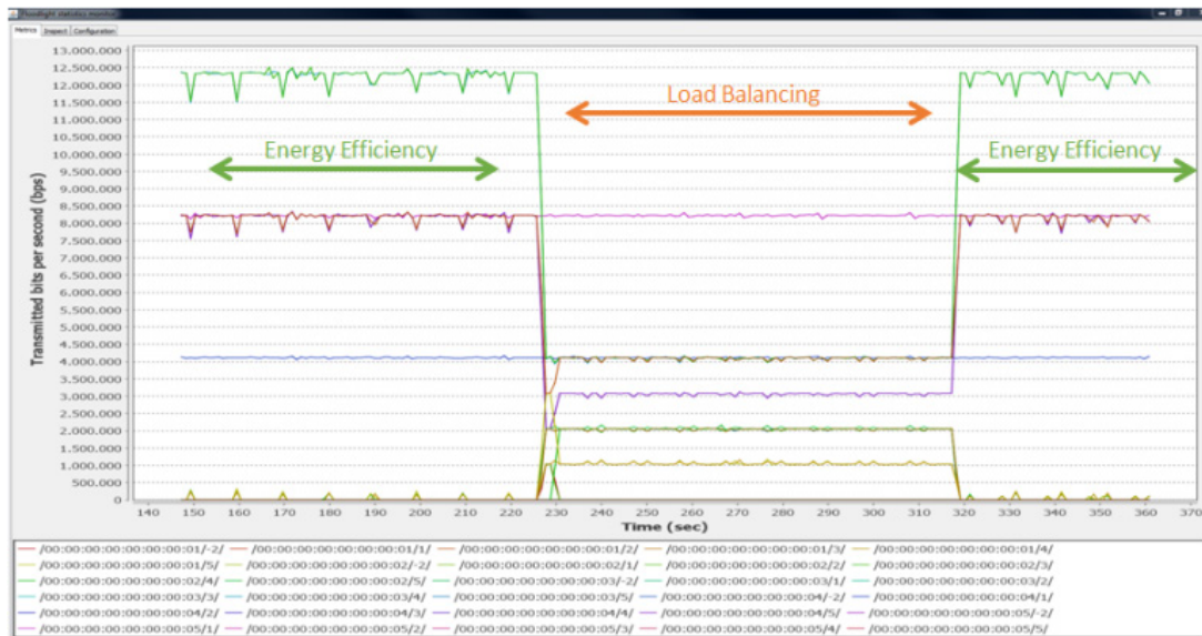
Figure 5-2: Transmitted bits per second for the two high-level policies (energy efficiency and load balancing), experimenting over the GÉANT OpenFlow facility.
