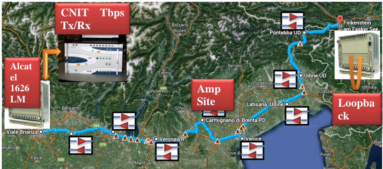
Figure 4.11 : The Field trial Setup
