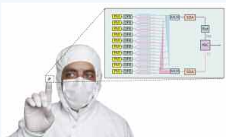
Figure 1. A fingernail-sized chip like this can deliver over 1Tb/s, and integrates around 300 optical functions. Each small box represents a discrete optical function that would otherwise be implemented in a separate module.
