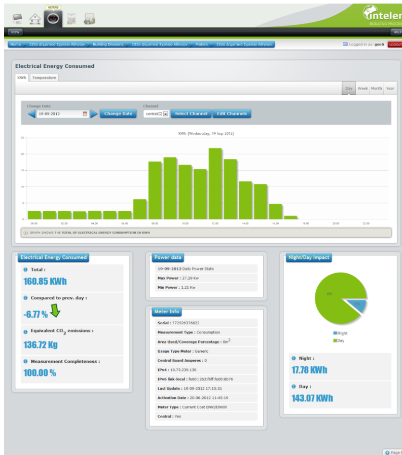
Figure 3: Real-time energy consumption data from a smart meter
