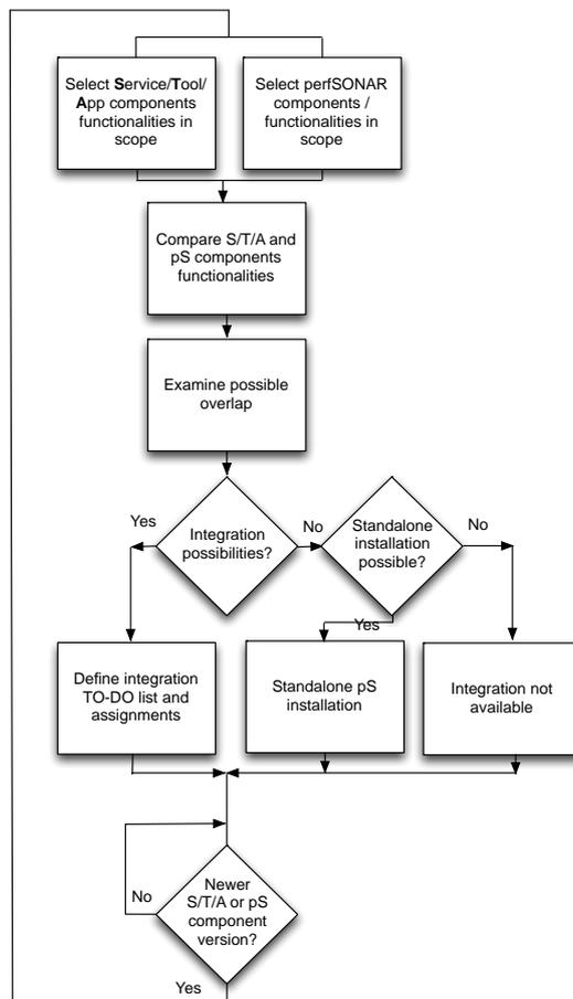
Figure 2.2: Model for Integrating perfSONAR for performance monitoring of other Services, Tools and Applications
