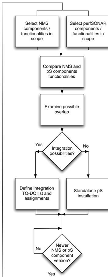
Figure 2.1: Model for integrating perfSONAR for NMS or perfSONAR component versions.
